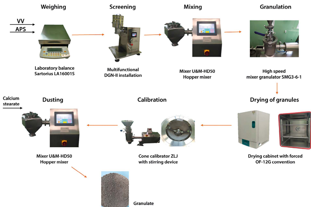
Figure 1. The granulation process mapping
