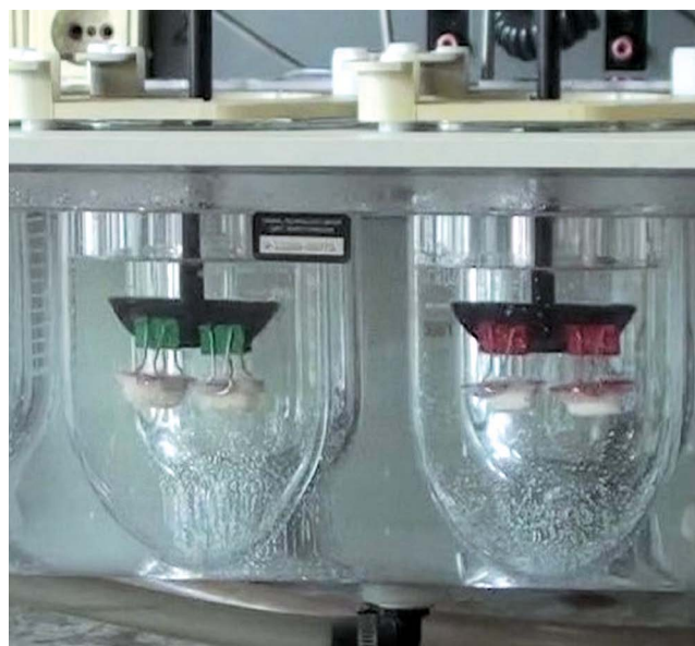
Figure 2. Control of swelling rate and duration of mucoaghesion of the tablets in dissolution type II apparatus
