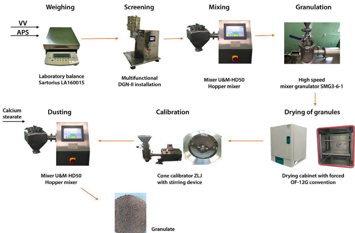
Figure 1. The granulation process mapping
